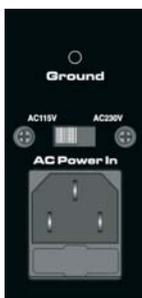
To connect the PM8 to your mains power source simply connect the included standard IEC mains power cable to the PM8's three (3) pin power connector socket.
